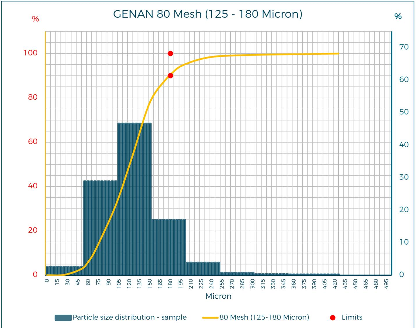
An Air Jet Sieve from Hosokawa Alpine is used to make a sieve analysis of the material / Test sieving in compliance with DIN ISO 3310-1.
